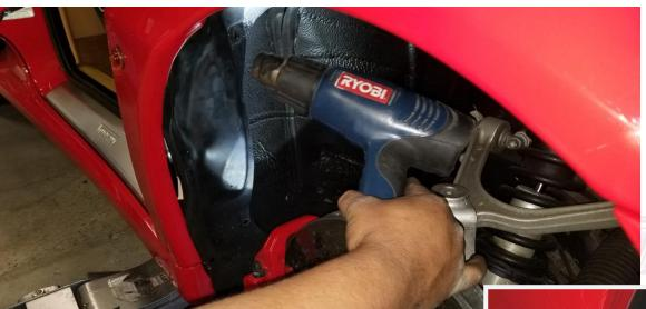
You will need to use a heat gun as shown to mold the splash guard to the back of the hinge.
