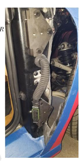
You will have to install the new VDI hinge to the spacers. Once the hinge is installed on the body of the car you will need two people to put the door up to the body and one person securing the 30MM bolts to the door.
