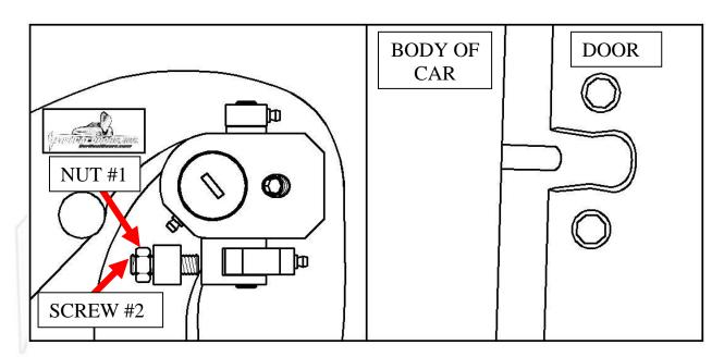
Note: You may need to slide the hinge forward or backward to make the hinge close properly.
