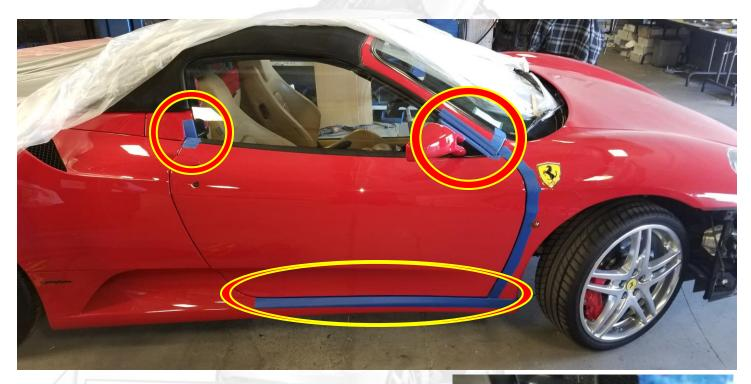
Remove the door by opening the door removing the door catch disconnecting the factory wire harness and removing the factory hinges.
