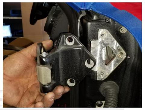
After removing the factory hinge you will have to installed the provided spacers. One spacer for the bottom and one for the top.
