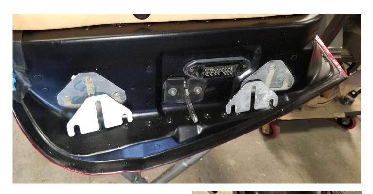
Once the door has been safely remove you will have to remove the door catch as shown.
